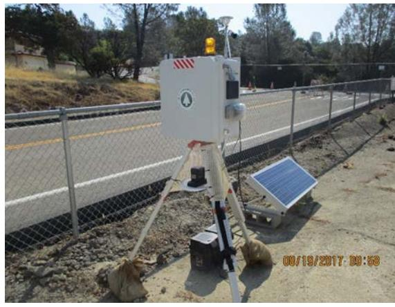
A photograph of an air monitoring station at Station 2. It features a white tripod-mounted control unit with a larger blue solar panel mounted on top, situated on a dirt area near a paved road. A chain-link fence runs along the background. The date "08/19/2017 09:59" is visible in the bottom right corner. |
