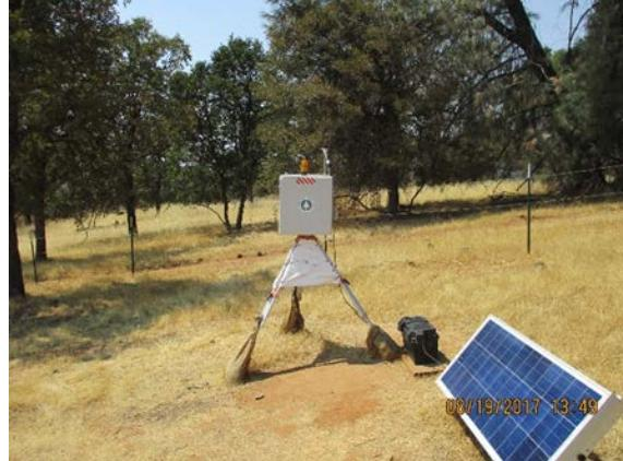
A white rectangular air quality monitoring unit mounted on a tripod stands in a grassy field. A solar panel lies on the ground to its right. The date '08/19/2017 13:49' is visible in the bottom right corner of the image.    |
