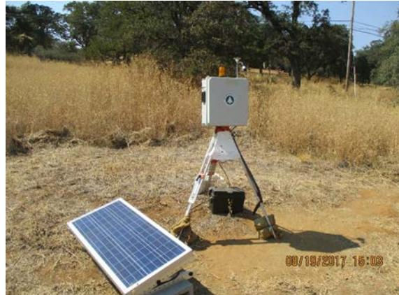
A white rectangular air quality monitoring unit mounted on a tripod stands in a dry, grassy field. A solar panel lies on the ground to its left. The date '08/19/2017 15:03' is visible in the bottom right corner of the image. |
