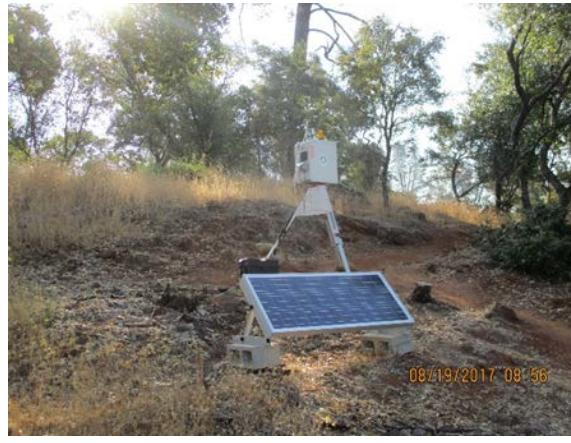
A photograph of an air monitoring station at Station 4. It is set up on a grassy, uneven terrain with trees in the background. The station has a white tripod-mounted control unit with a blue solar panel. The date "08/19/2017 09:56" is visible in the bottom right corner.                                    |
